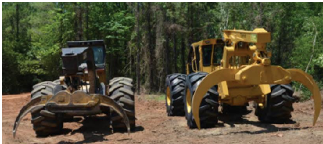
Figure 31. Conventional (left) and high-capacity grapple skidder (right) for transporting small diameter pulpwood from the forest to the landing. Photo credit: Auburn University High Tonnage Forest Biomass Project 58 .
