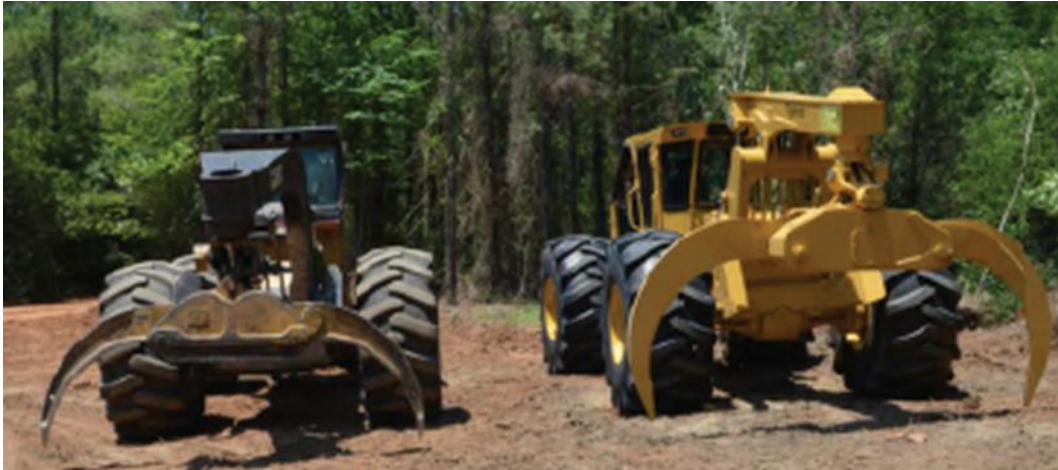
Figure 35. Conventional (left) and high-capacity grapple skidder (right) for transporting small diameter pulpwood from the forest to the landing. Photo credit: Auburn University High Tonnage Forest Biomass Project 58 .
