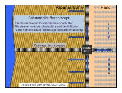
The water quality challenge of reducing nitrates from tile drained cropland was already noted. This schematic shows a saturated buffer designed to remove nitrate mainly through microbial denitrification. The saturated buffers now being tested by the Agricultural Drainage Management Coalition through a USDA Conservation Innovation Grant are installed in CRP buffers.
